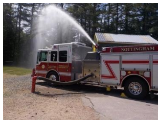
Testing the fire hydrant
